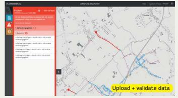
Data on sewer infrastructure in ingested in a central database using Aquastreng2.1 Data is validated according to topological and functional requirements
