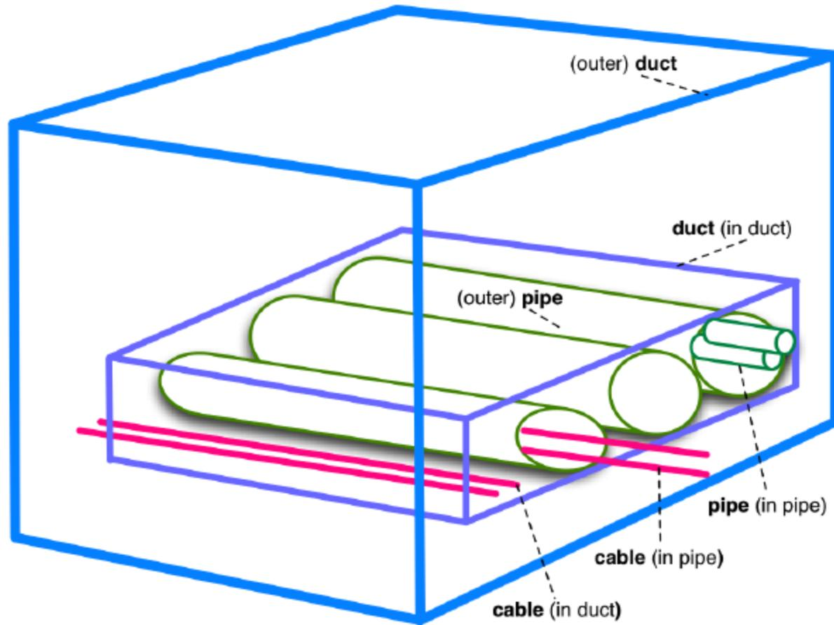
Figure 9 – Physical relations between cables, pipes and ducts
