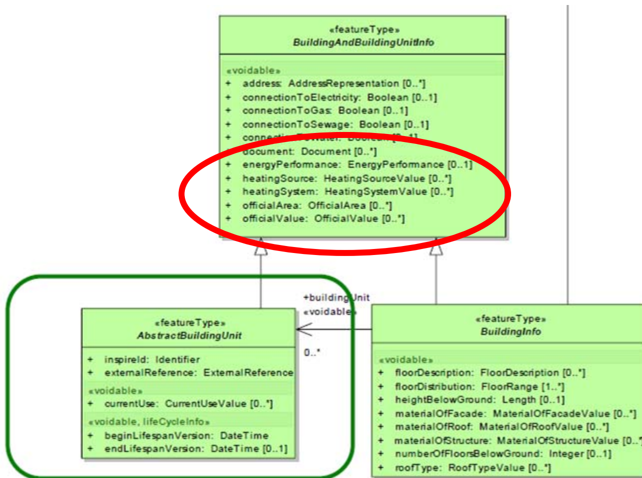
Figure 37: Main feature types of Buildings Base Extended
